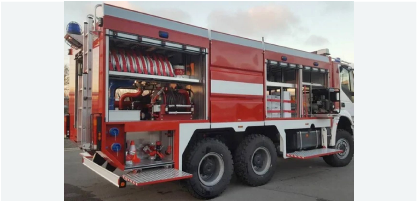
Fire engine with open equipment compartments, hoses and equipment components.
